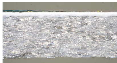
Figures 61 and 62 – Carbon and Carbro. Cross-sections in a 200x view, with BF reflected lighting (left to right). Both prints have a baryta coating to separate the gelatin layer from the paper support. In the Carbro example, the color layers are tightly overlapped.
