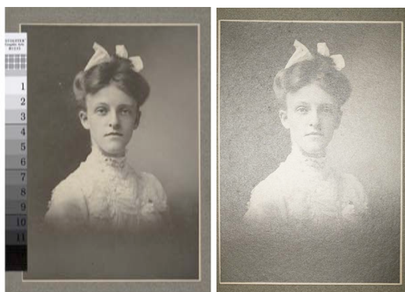
Figures 48 and 49 – Matte collodion POP print. Normal view at 45° and 0° lighting (left to right). Unlike the collodion P.O.P. print, the surface isn't glossy, because light is being scattered by the surface irregularities.
