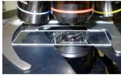
Figure 129 – Placing the glass slide under the microscope for observation of the cross sections.
