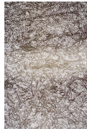
Figure 121 – Matte collodion print at 50x magnification, seen under non polarized BF (simulating 0° lighting). The surface has many irregularities for the light to interfere with.
