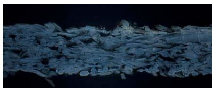
Figures 149 and 150 – Engraving and etching (left to right). Cross sections at 200x, with BF reflected light and DF-UV light. The paper fibers show no fluorescence.
