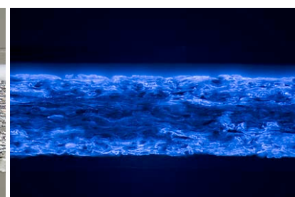
Figures 99 and 100 – Inkjet print (dye) on a swellable support. Cross-section at 200x with BF reflected light and DF-UV light (left to right). The RC backing and front layer cause this fluorescence.
