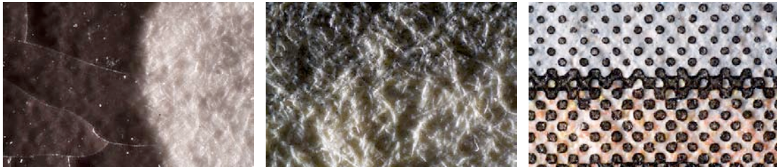
Figures 31-33 –Woodburytype, rotogravure and letterpress halftone prints (left to right). 50x view at 90° lighting. Fibers are visible on the non image areas of the Woodburytype, all across the rotogravure surface, and hidden in the letterpress halftone print, due to an extra coating.
