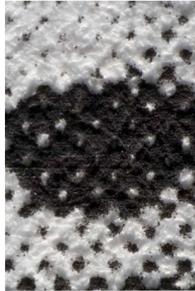
Figure 80 – B&W electrophotographic print. 50x view at 90° lighting. The dusty quality of the print can be seen.
