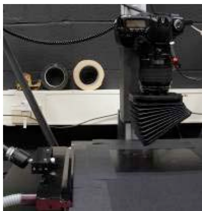
Figure 113 – Copystand setup for the racking light shot. The fiber optics cable is on the bottom left
