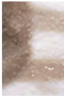
Figures 160-161 – Agfacolor, Cibachrome (left to right). 50x view at 90° lighting. Using a plastic coating over a paper base core prevents the print's surface from showing irregularities related to those fibers.
