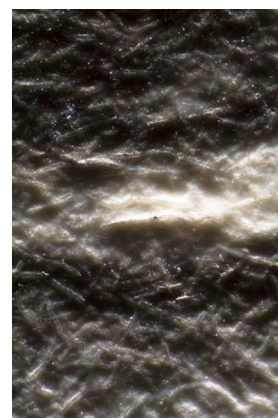
Figure 50 – Matte collodion POP print. 50x view at 90° lighting. Because the image has a thin baryta layer, its possible to observe paper fibers.
